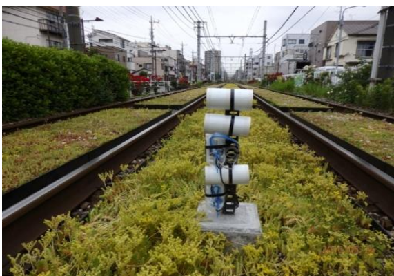
Photo.5 Arranged temperature sensor (left:Orbid greenery, right: Ballast in an orbit)
