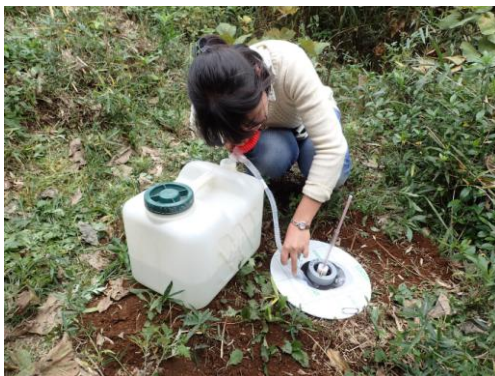
Photo.8 Measurement of water permeability (left) and soil hardness (right)
