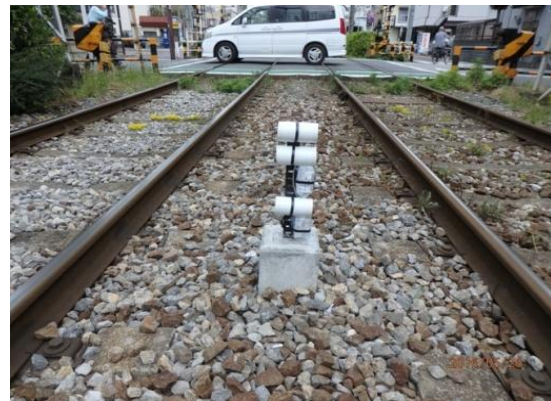
Photo.5 Arranged temperature sensor (left:Orbid greenery, right: Ballast in an orbit)
